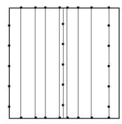
4. Draw straight, vertical lines from each mark on the top of the square to the mark directly opposite it on the bottom of the square.
