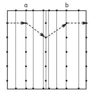
5. Mark a line ('a') about 4 spaces left of the centre. Mark a matching line ('b') on the right of the centre. Mark spaces to match the spaces on the side of the square. Draw horizontal lines across the square to connect the marks on either side. When you get to the 'a' line change the angle and draw a diagonal line down to the mark one space lower on the centre line. When you get to the centre line change the angle again and draw a diagonal line to the mark one space above the centre line.
