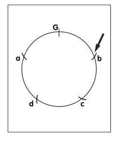
6. Keep the radius of the compass the same. Move the compass point to **b**. Draw a new short arc that intersects the circumference at **c**. Move the compass point to **c**. Draw a new short arc that intersects the circumference at **d**. Erase the construction lines.
