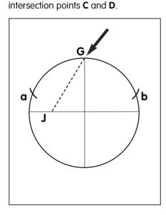
5. Set the radius of the compass the length of GJ. Place the point of the compass on G. Draw 2 short arcs that intersect the circumference on the left and right – a and b.
