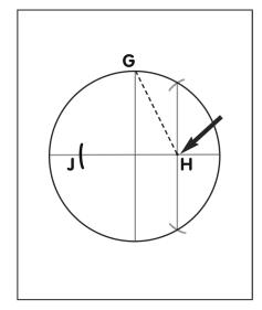
4. Set the radius of the compass the length of **GH**. Place the point of the compass on **H**. Draw a short arc that crosses the horizontal diameter on the left – **J**.
