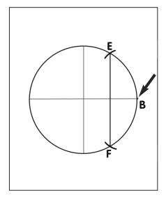
3. Set the compass to the radius of the original circle. Place the point of the compass on point **B**. Draw 2 short arcs that intersect the circumference of the circle – **E** and **F**. Draw a vertical line that connects the intersection points **E** and **F**.
