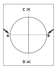
2. Enlarge the radius of the compass. Place the point of the compass on point **A**. Draw a short arc above and below the circle. Keep the compass open at the same radius. Place the point of the compass on point **B**. Draw short arcs above and below the circle to intersect the other arcs. Draw a vertical line that connects the
